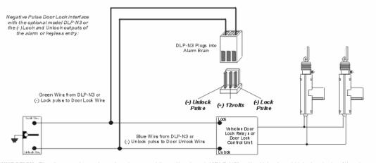
CONNECTION: The diagram above shows how to connect the optional model "DLP-N3" or the (-) Lock and Unlock outputs of the alarm or keyless entry to a Negative Pulse type door lock system. If the door lock system requires more than the 250 ma. door lock outputs from the alarmor keyless entry, then use the diagrambelow to wire the optional model "DLS" to the door lock system in the vehicle.
