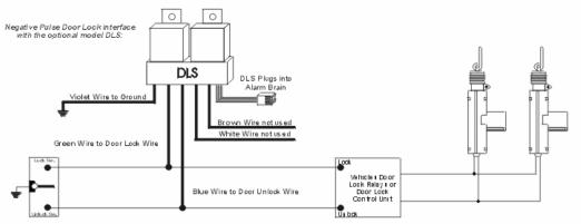
**CONNECTION:** The diagram above shows how to connect the optional model "DLS" to a Negative Pulse type door lock system. If the relay s are going to be wired directly without the optional model "DLS", then use the "DLS" wiring diagram NOTE #200 to see how the relay coils are wired to the alarm brain outputs & how the wires from the relay contacts are wired to interface with the door lock system.
